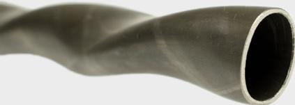
When standard ECT probes are inserted in Twisted Tubes®, the probes cannot provide reliable data because the flaws on the wall furthest from the tube's center (crest) produce much weaker and distorted signals compared to same-size flaws in the narrow section, closest to the tube's center (dip). This is because of the liftoff created by the tube's geometry between its walls and the ECT probe. This amount of liftoff translates into a lower probability of detection and less accurate sizing.
