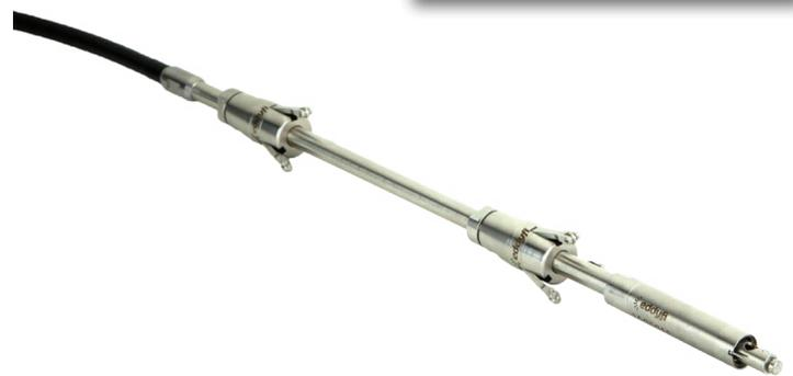
The Eddyfi IRIS inspection solution features patent-pending impedance matching, which can reduce the defect detection limit to 0.8 mm (0.03 in), increasing the detection limit to approximately 80% of the tube thickness, making sizing deep defects in thinner tubes possible.
